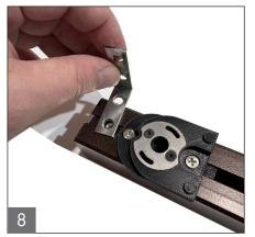
With rod installed in place, open the lever on the motor.
